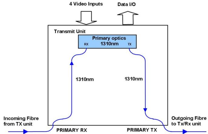
The **AMG3743Bx** receives and drops off data signals transmitted from an **AMG3784Bx** receiver. It then inserts video and data signals onto the outgoing optical signal.
