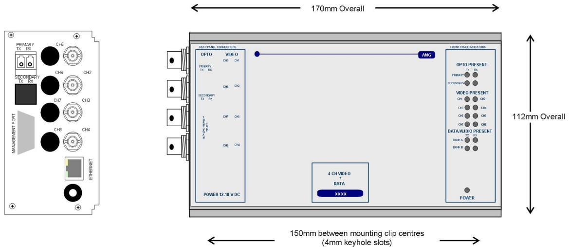
The **AMG3743Bx** is a standalone four channel video insert unit designed to transmit 4 video signals and transmit & receive 2 bi-directional data channels to/from a singlemode optical fibre ring.
